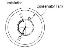
Installation measure acc. with DIN 42569
