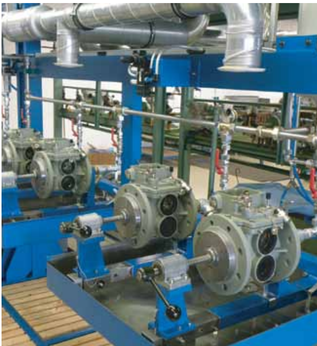
Figure 10 - Functional and leakage test
